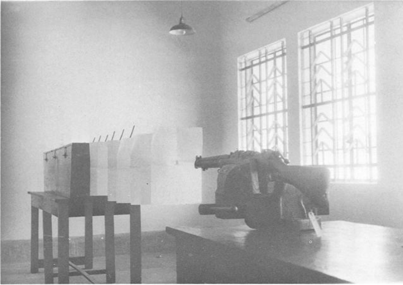
FIG. 2—Experimental arrangement showing the 0.410 musket and paper screens (0.013 cm thick) in front of bullet recovery box.
